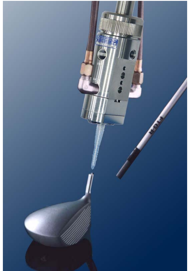
Mix-Dispense Valve position when placing adhesive in hosel
