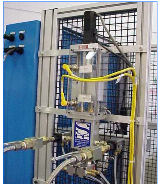
Servo-Flo 801 Meter and Panel Assembly are fence mounted using a remote mounted 2200-545 Mix Dispense Valve (not shown)
