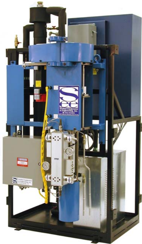
Frame mounted ISD Meter integrated with Heat/Cool Temperature Conditioner
