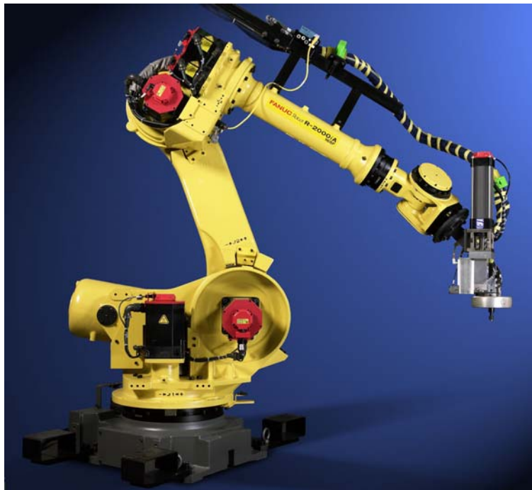
FANUC Robotic Dispense System with KISS Valve Applicator and Vision System. Dispenser, Tooling and Dress-Out Engineered by Sealant Equipment & Engineering
